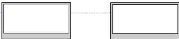
Fig 6 Dual pontoon floating breakwater
